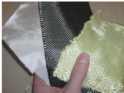
Figure 2: Woven Glass (white), Carbon (black), and Kevlar (yellow) fibers clothes.
