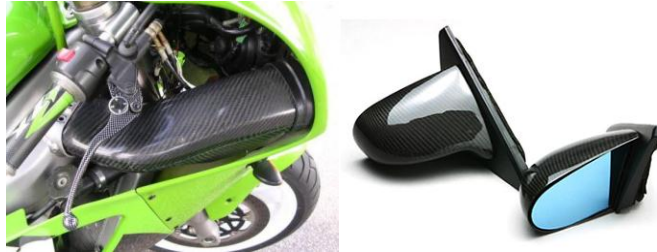
Figure 4: Carbon fibers air duct and a break handle on a motorcycle (left) and a side mirror cover made of carbon reinforced epoxy (right)
